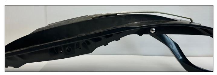
2.2 Mark on the ski each side of the folded end of the Trek runner. Remove the runner.
