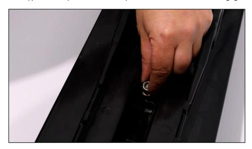
2.9 Using a ratchet, tighten the nuts starting with the center nut, tightening all the bolts until the runner tightens on the ski. Refer to the tightening torque according to the nuts supplied with the product.
