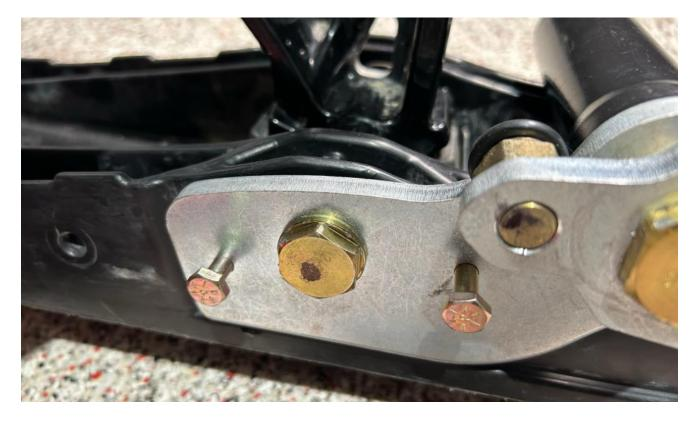
Insert nuts [P7] on safety bolts [P6]. Torque to specified torque. 3.23.
