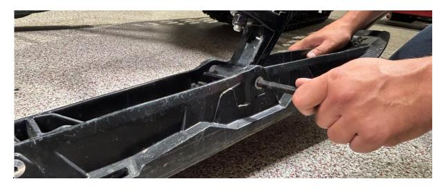
3.4. Remove ski axle from the leg and the original spacers. Set the original spacers aside.
