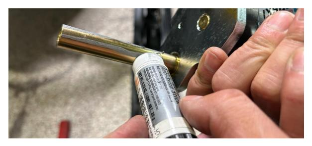
3.15. Insert the shim [P9] into the RollerSki axle. Pre-engage the RollerSki axle in the ski, put the washer [P5] from the hardware removed earlier. The washer is used to replace the bushing removed in step 3.5 of vehicle preparation.
