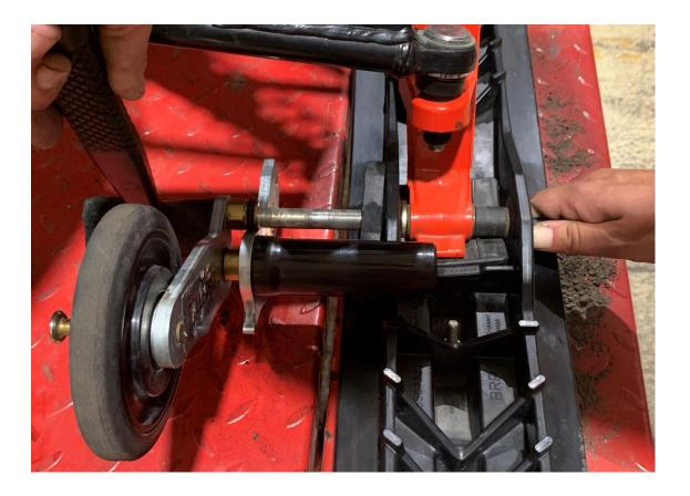
3.19. Apply red Loctite 263 to the threads of the bolt [P3].
