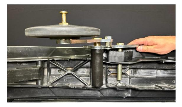
3.8. Temporarily screw the bolt [P3] into the axle for added stability.
