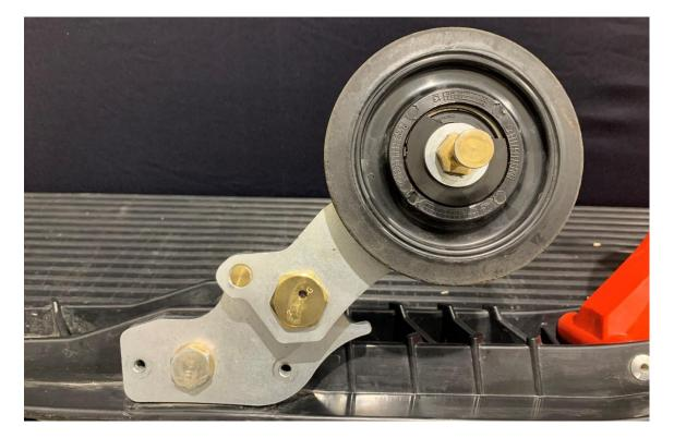
3.10. Using the holes in the base of the RollerSki as a guide, drill the shoulder of the ski with a 1/4" drill bit. Drill only the side where the RollerSki is installed.
