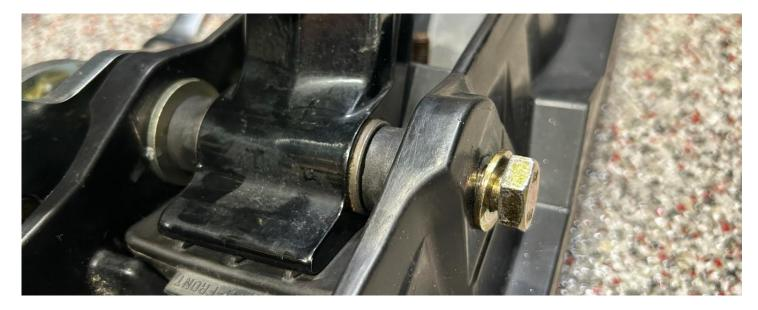
3.21. Tighten the bolt [P3] in the axle. Tighten to specified torque.
