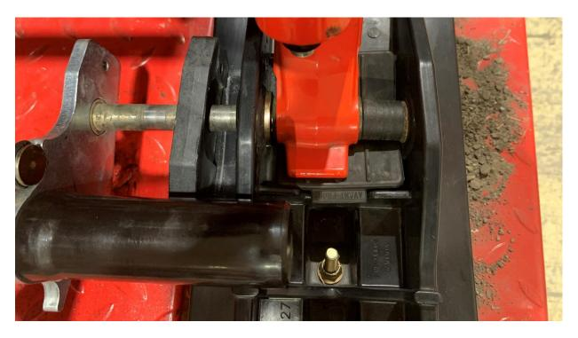
3.17. Take the original screw removed in step 3.3 of vehicle preparation and insert it through the ski, spacer and ski leg up to the RollerSki axle. Tighten by hand. This will make it easier to pass the axle through the ski leg
