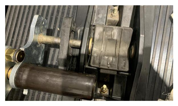
3.16. Position the ski under the ski leg and lift the front of the ski to keep pressure on the assembly. Make sure that the holes in the ski and the ski leg are well aligned and that there is enough space to put the second original spacer. Lower the snowmobile onto the ski rubber.
