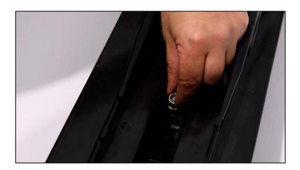
3.3 Using a ratchet wrench, tighten the nuts starting with the center nut, tightening all the bolts until the runner is snug against the ski. Refer to the torque specifications according to the nuts provided with the product.
