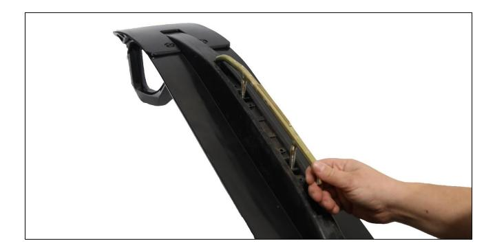
3.2 Insert the nuts onto the studs and tighten by hand
