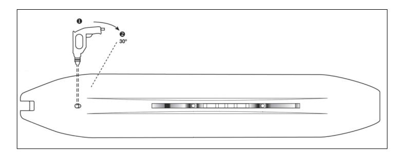
3.7 Insert the front of the runner into the hole drilled in the ski in the previous step. Rotate the runner to align the studs with the holes in the ski. If necessary, use a rubber mallet to position the runner in the ski.
