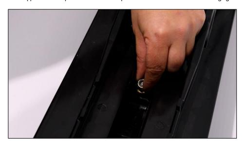
3.9 Using a ratchet, tighten the nuts starting with the center nut, tightening all the bolts until the runner tightens on the ski. Refer to the tightening torque according to the nuts supplied with the product.
