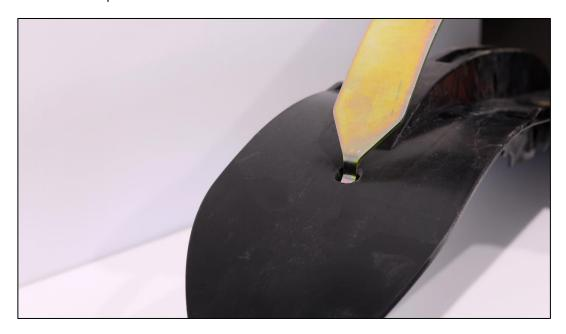
3.8 Insert the nuts onto the studs and tighten by hand
