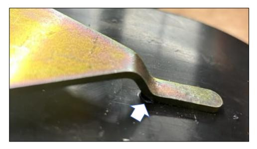
3.6 Using a  $\frac{1}{2}$  " drill, drill the hole made previously and tilt at 30°.
