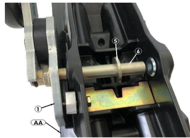
\*\* THE WASHER (#5) WILL REPLACES THE BUSHING REMOVED AT STEP B.
