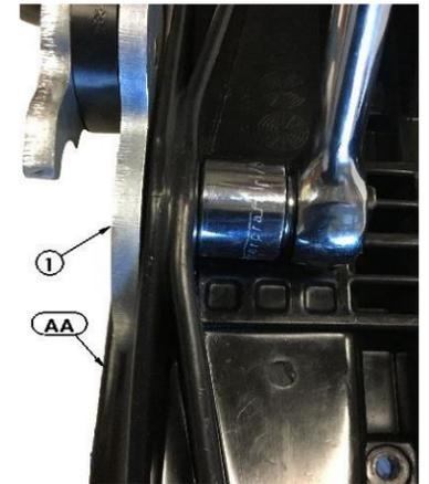
\* **THE SOCKET (#2) WILL REPLACE THE BUSHING REMOVED AT STEP B.**
